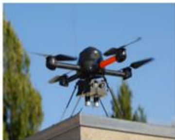
Figure 5: Quadcopter micro UAV 'microdrones md4-200' with the prototype MSMS multispectral sensor. Nebiker et al., 2008
